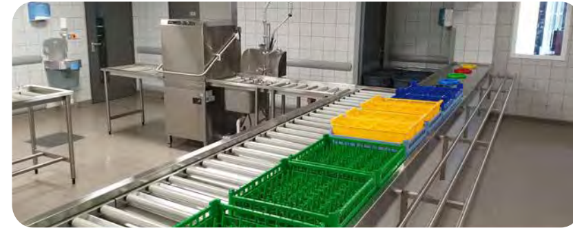
Pass-through machine with automatic hood-lift system
