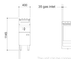
The unit can be connected at the rear or from below
