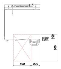
If a Gully is used in the premises, ensure it covers the highlighted area.
