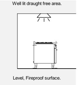
**CAUTION:** If suiting, the necessary clearances to any combustible wall **MUST BE** the largest figure given for individual appliances instructions.
