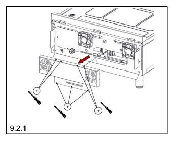
9.2.1 To remove undo screws on the rear fan cover to release panel.
