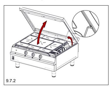
9.7.2 Tilt hob up and lift hob stay into position. Insert cranked end into slot on underside of hob.as shown above. Ensure stay is secure before work is carried out.
