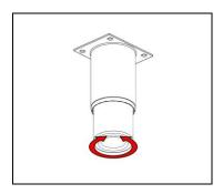
8.2.3 When on stand to adjust height of unit with feet twist lower half of feet as necessary.
