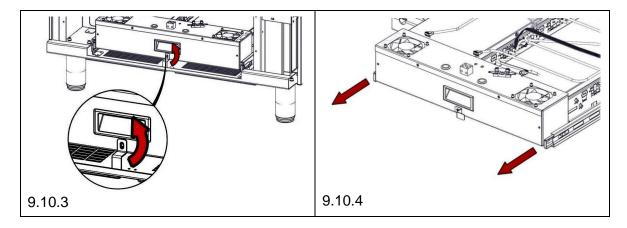
9.10.5 Gently slide out generator tray ensuring not to snag any cabling within the unit.
