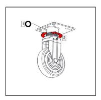
8.2.4 To adjust height of castor, loosen grub screw and twist body of castor as necessary.
