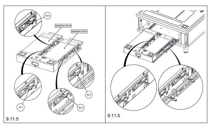
9.11.6 When re-fitting ensures all electrical connections & memory sticks are restored as detailed in the wiring diagram.
