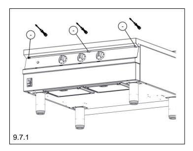
9.7.1 Remove fixings at top control panel.
