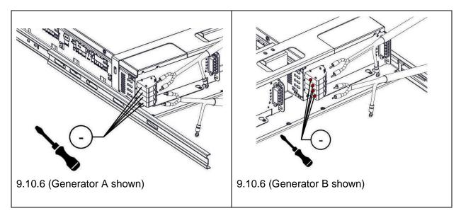
9.10.7 When re-fitting ensures all electrical connections are restored as detailed in the wiring diagram.
