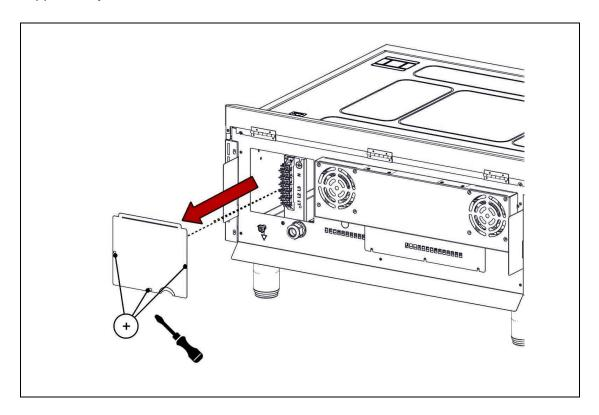
To install the mains cable, remove terminal cover and feed the cable through the cable gland and connect the mains supply to the terminal block.
