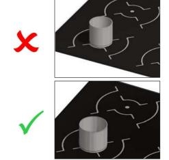
Figure 3 Unit will not Operate
